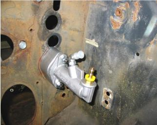
2.3 Verify actuation of the lever assy with master cylinder attached. The master cylinder will have 1.4" of total travel. Verify master cylinder does not bottom out on lever and that lever does not contact the cap screw. Install e-clip on clevis pin. Tighten the hardware as shown using a 1/2" wrench/ratchet. Verify the clutch pedal rests against the stop when adjusting rod-ends.
